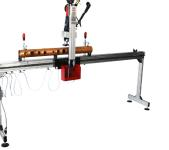
Manually operated unit for use in conjunction with the T-DRILL T-35 or T-65 collaring machines in small volume production of copper and aluminium manifolds. Produce twenty 28 mm collars in less than ten minutes without moving the tube.
