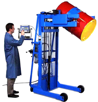
Scale-equipped to dispense measured amount from drum
