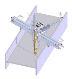
The H Beam system is designed with a track mounting device which uses on/off magnets on a swivel hinge to provide both linear and angular cuts. The mounting device is unlocked which allows the track to swivel on its axis. This is ideal for applications which also require cuts to be made on a 45° angle for butting two beams together.
