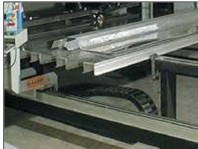
Longitudinal track and cables are located underneath the table in protection.
