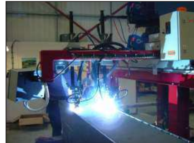
Gullco Gantry system is equipped with dual torches enabling simultaneous welds on both sides of aluminium trailer sidewall stiffeners in one pass.
