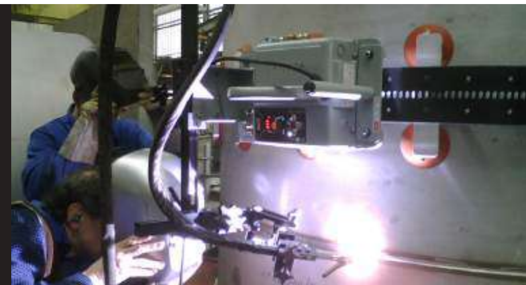
G. 4 MOTION SEMI-AUTO GUN HOLDER Mounts on the KAT® horizontal rack arm to provide 5" (127 mm) of vertical adjustment 360° torch rotation & two directional angle tilt
