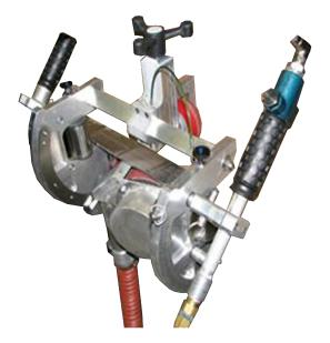
The PRC is a carriage which utilizes an aggressive belt mount on a Gullco customized automation carriage. This unit is used to remove surface rust and pre-construction primer from steel plates several times faster than manual processes while also reducing the change of potential injuries and fatigue.
