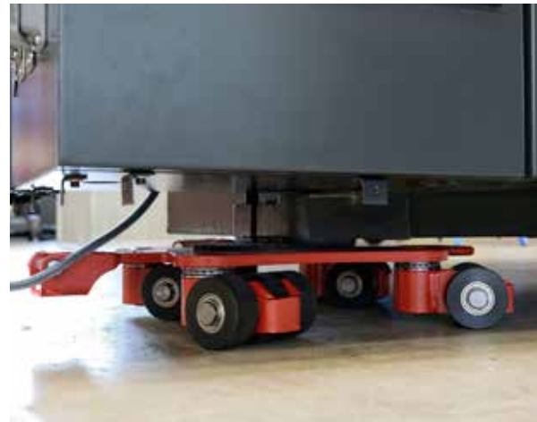
Revolving trolley JKB in action
