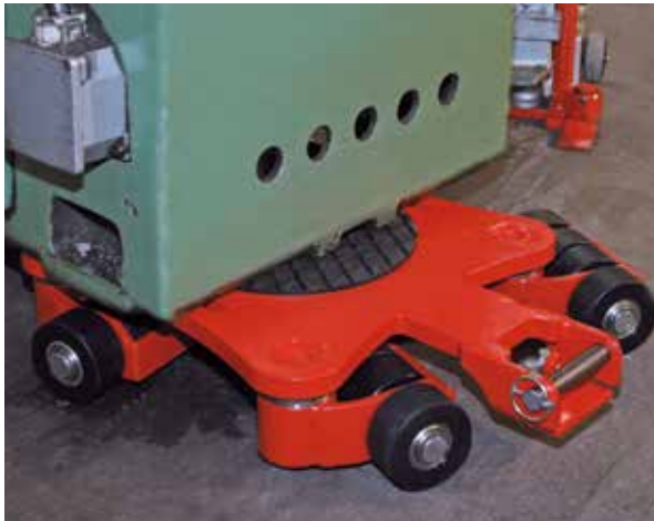
Revolving trolley JKB in action.
