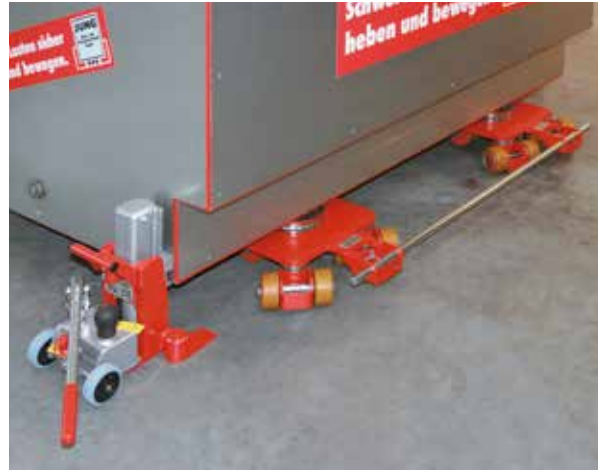
Example as adjustable trolley
