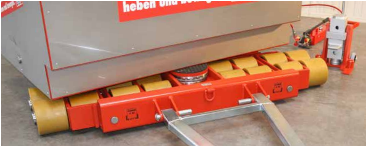
Steerable H-series trolley in action
