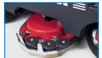
Swivelling brush head allows cleaning close to the edge
