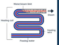
The water flows through the heating coil and is heated by the heating wire. Before exiting, the water turns into steam and can be pumped on to the consumer.
