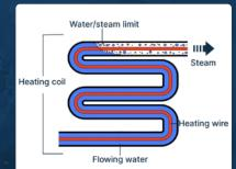
The water flows through the heating coil and is heated by the heating wire. Before it exits, the water turns into steam and can be pumped on to the consumer.
