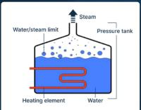
Heating elements in the water cause it to evaporate under pressure. The steam is led upwards to the consumer.
