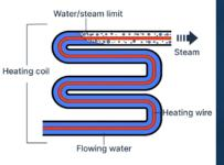
The water flows through the heating coil and is heated by the heating wire. Before exiting, the water turns into steam and can be pumped on to the consumer.
