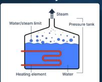
Heating elements in the water cause it to evaporate under pressure. The steam is led upwards to the consumer.
