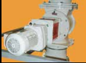
Rotary valve discharges the collection container continuously
