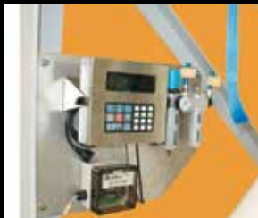
Electronic scale controls the filling weight of the BigBag
