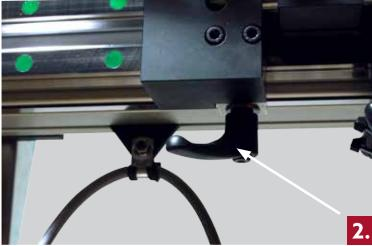
2. Free positioning with locking lever and measure.
