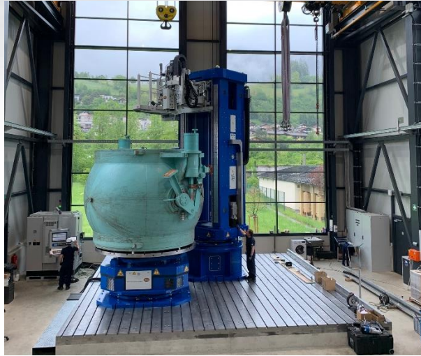
Mobile machining center (MMC) for turbine housings for hydro energy
