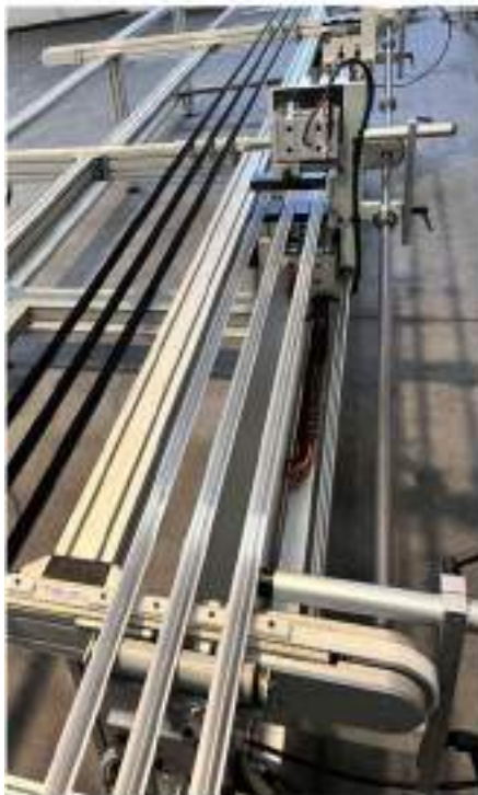
Specially designed GAA-350 Machine with automatic profiles loader for three bars processing simultaneously
