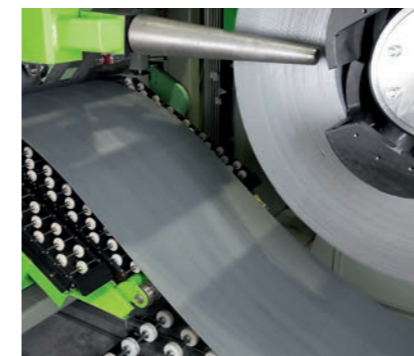
— Strip threaded into levelling machine
