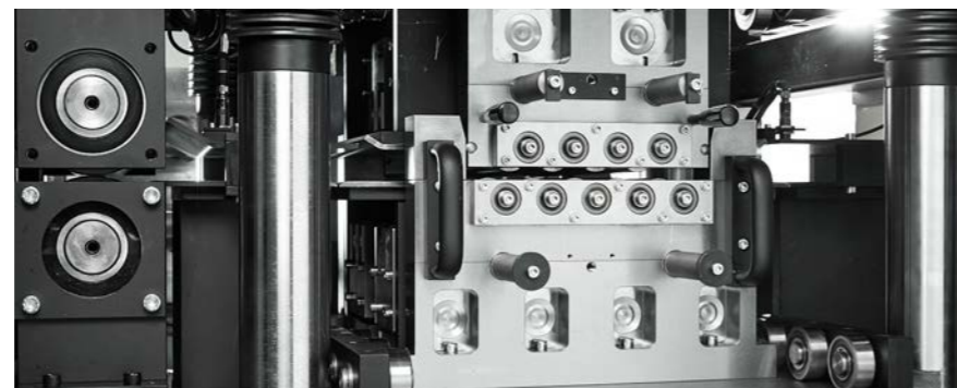
— Strip take-off with levelling unit
