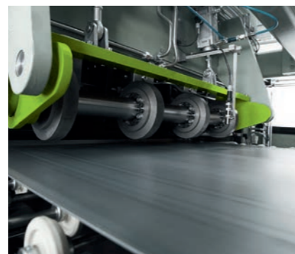
— Strip levelling machine in compact design
