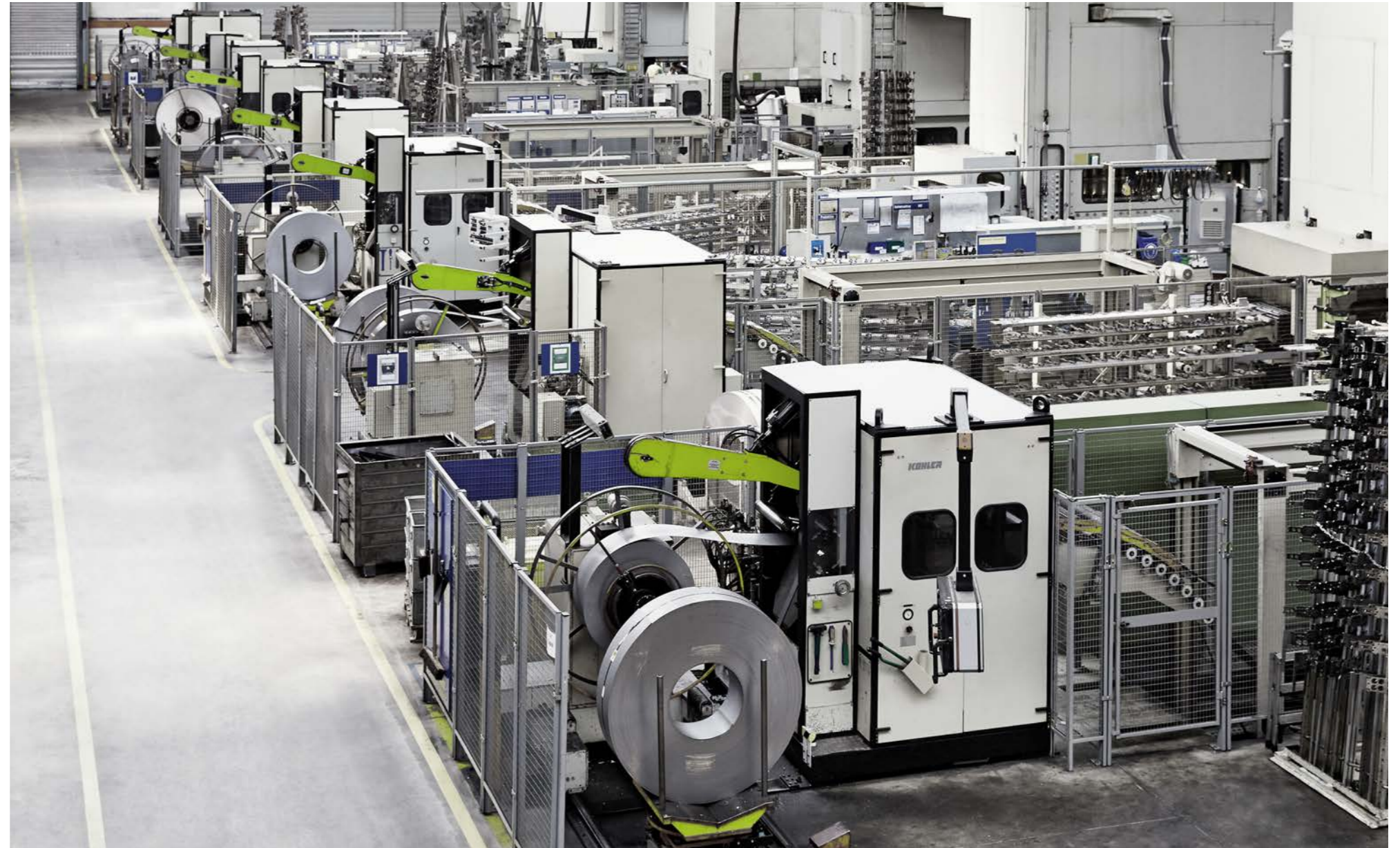
— KOHLER strip levelling units in several production lines of a regular customer
