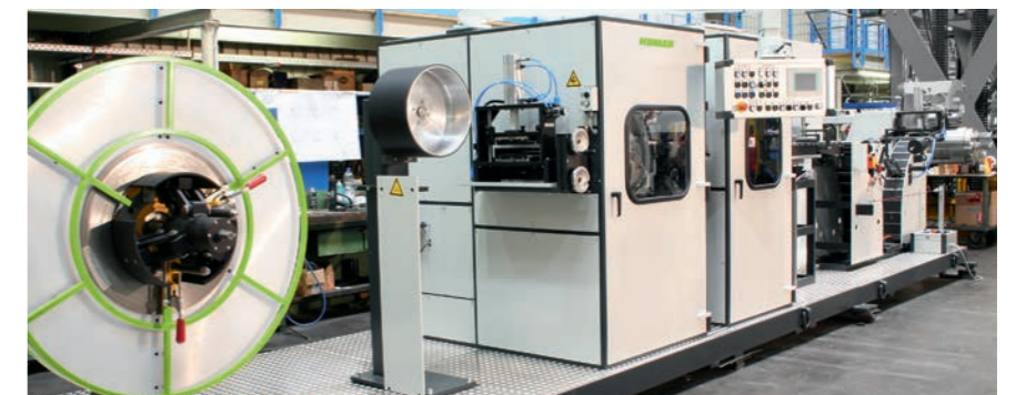
— Recoiling line with camber levelling technology
