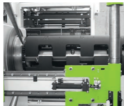
— Coiler with toothed rack expansion
