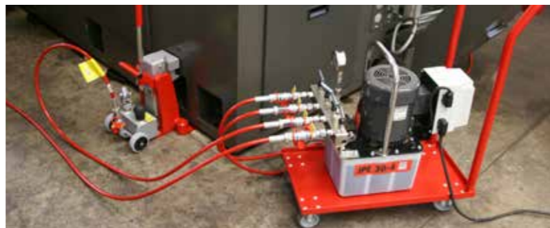
Electric pump JPE 30-NVR with 2 jacks in operation.
