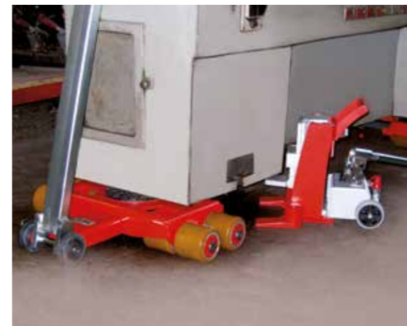
Castors with ball bearings guarantee easy movement.
