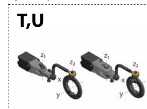
T: from 0 up to 15 kg with Quick change X:Turns 360°. Lockable 4x90° Y:Turns 360° Z1:Turns 90° right & left Z2:Turns 360° U: from 15 up to 30 kg X:Turns 360°. Lockable 4x90° Y:Turns 360°. Lockable in any position Z1:Turns 90° right & left Z2:Turns 360°
