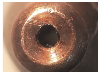
Fig.2 Contact tips outlet hole wear after 30 minutes of pulsed MAG welding. 240 A, 29 V.
