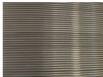
Fig.1 Surface appearance of INEFIL NR 1.2 mm after an 88-hour exposure in a climatic chamber at 35°C and 95% humidity (tropical conditions).
