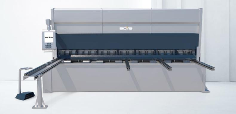
Strips are less twisted when cutting thicknesses less than the nominal thickness, by using a smaller cutting angle.
