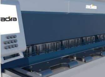
Robust back gauge with movable positioning, allows rotation for retraction of the guide
