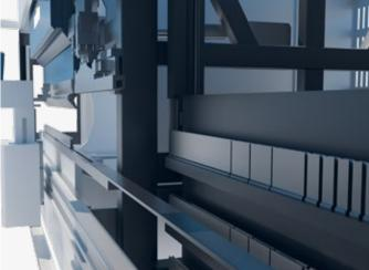
Manage the tools needed for bending. The system selects and positions the tools and dies available in the automatic tool warehouse, avoiding the manual selection and changing of tools and dies
