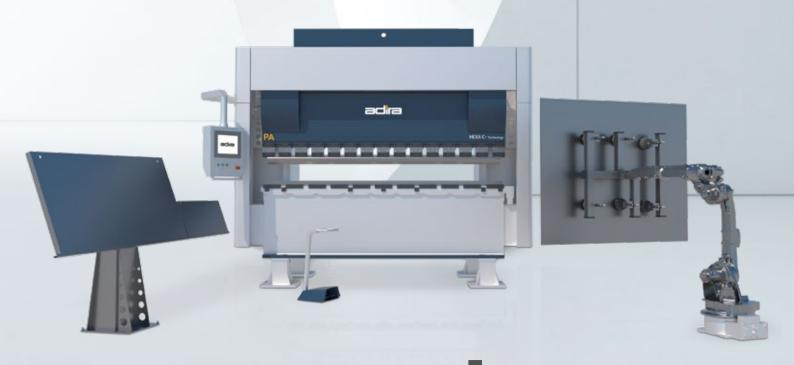
Other kinds of operations in addition to the manufacture of bent parts can be added to the cell and carried out by other machines, such as sanders, small punches or welding machines operated by the same robot.
