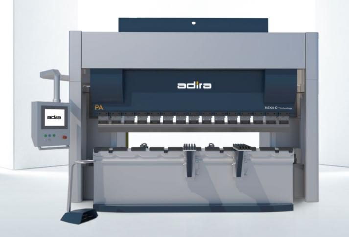
The HEXA-C® frame ensures better bending precision, given that the movable ram stays perfectly aligned with the fixed ram.
