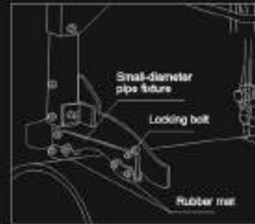
Small-diameter pipe fixture (optional)
