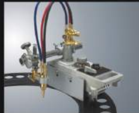
Circle cut w / circle rail
