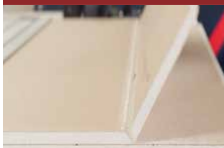
V-shaped grooves for folding/bending technology (90° + 45°)
