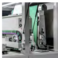
Upper deburring and edge rounding station
