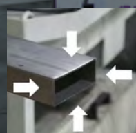
FGW170 8Z: Finishes all four sides simultaneously
