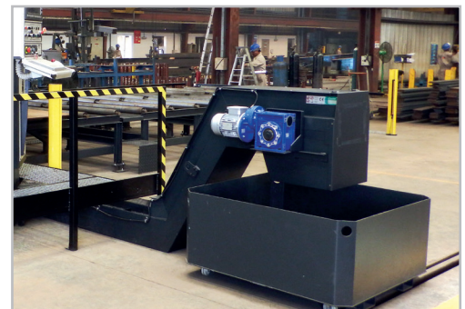
Chip and small pieces extraction belt Cinta extractora viruta o pequeñas piezas
