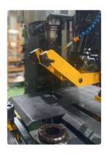
**DRILLING UNIT**9kW Drilling unit up to 40mm diameter.
