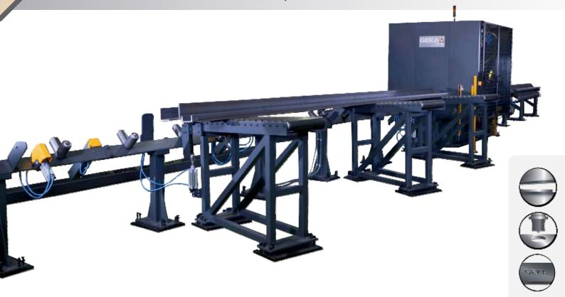
The **GR series** are machines designed for maximum output and processing quality in the minimum space possible. The material is moved by means of a roller to optimize efficiency in a reduced space. Though the material is moved by a **roller infeed**, the customer can use GEKA's patented **Minimal Waste System** to ensure a minimum waste per bar, **reducing the scrap to virtually zero**.
