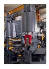
MITRE SHEARING FOR FLATS Maximum turning capacity +/- 45°.
