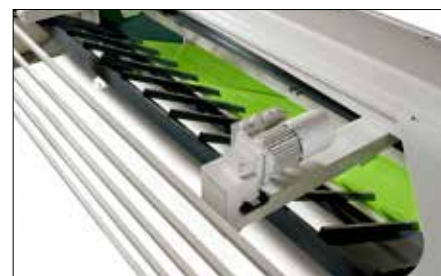
Sheet support in lower position for delivery of cut-off material to the front, operation controlled from CutLink.
