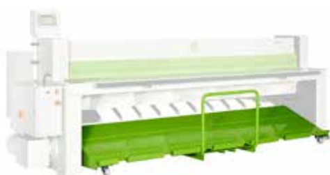
With a wagon as an alternative to fixed return plate you easily transfer cut material to another work station.
