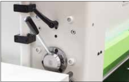
Simple and clear blade gap adjustment for varying thicknesses.
