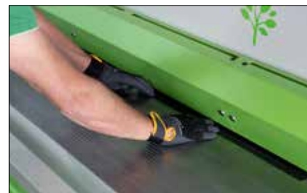
Hold down beam only 32 mm (1.25") from the cutting line for minimal waste.
