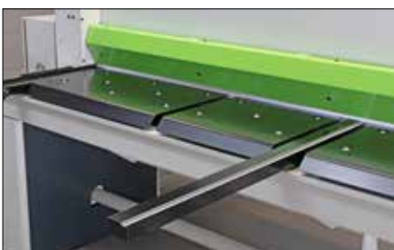
The strategically positioned support arms facilitate handling. Cut piece support at the front of shear with T-groove and tilting stop, means the trimmings remain inside the machine.
