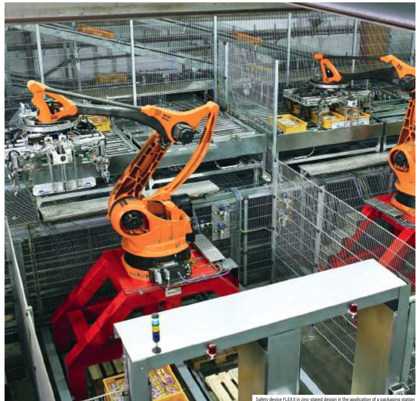
Safety device FLEX II in zinc-plated design in the application of a packaging station
