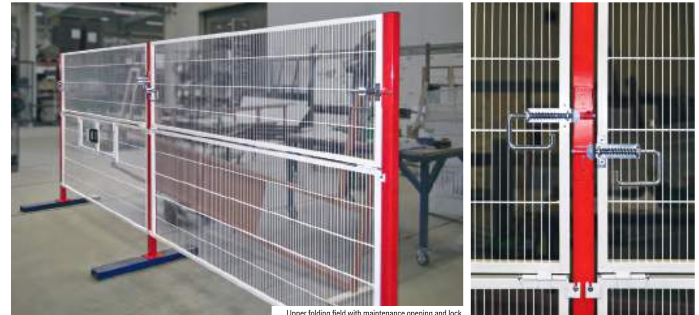
Upper folding field with maintenance opening and lock
