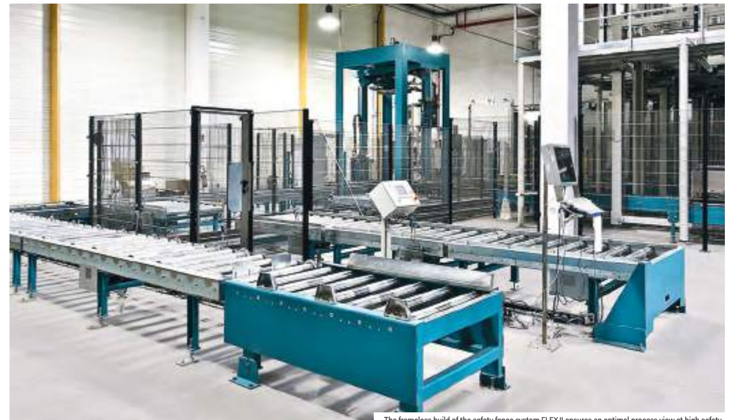
The frameless build of the safety fence system FLEX II ensures an optimal process view at high safety
