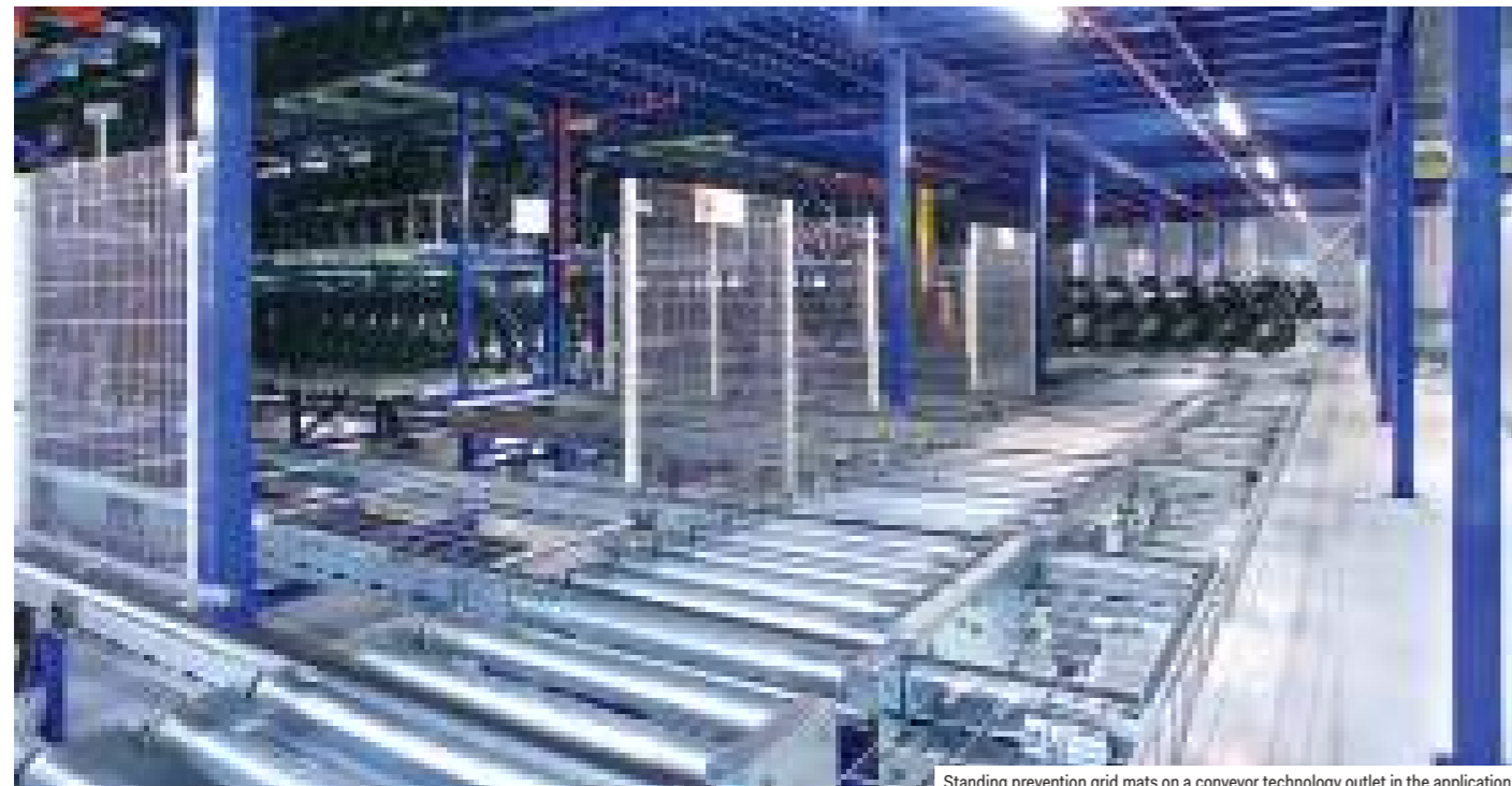
Standing prevention grid mats on a conveyor technology outlet in the application
