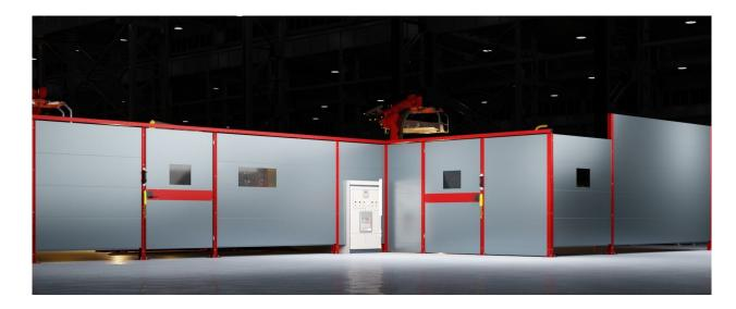
The Eye Safety Fence (ESF) protective fence system is characterised by its versatile applications. One example is in welding and laser processing lines, especially on a larger scale, as well as processes that require high safety standards. The system is offered in two standard heights (2200 mm and 2700 mm) but can be customised according to project requirements if needed. The ground clearance of 180 mm can be reduced to 20 mm with the ground element.
